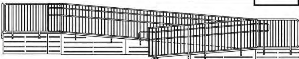
5 HI U-TURN RAMP W/2 INTERMEDIATE LANDINGS TO ACCESS UP TO 35" IN HEIGHT.
